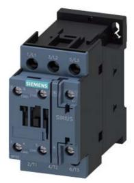
CONTACTOR, AC-3, 18.5KW/400V, 1NO+1NC, AC 230V 50HZ, 3-POLE, SZ S0 SCREW TERMINAL
